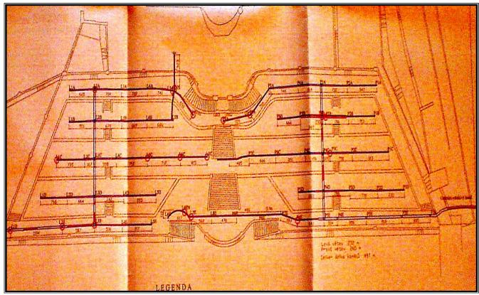
This plan illustrates how the individual channels in the western garden are interconnected. This documentation comes from a survey of the garden terrace drainage conducted in 2004.
